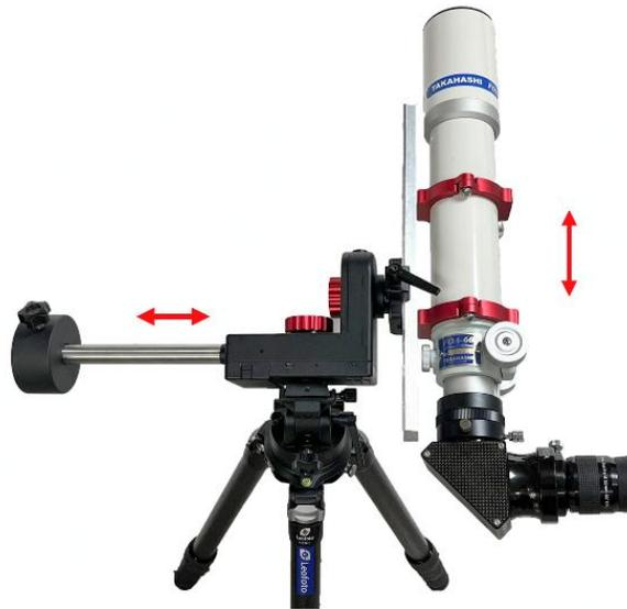
Figure 13 Balancing a telescope
