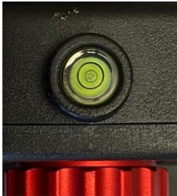
Figure 17 Leveling a SkyHunter in AA mode
