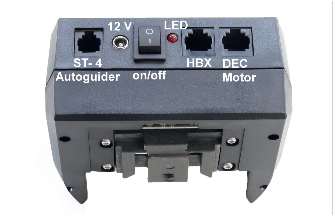
Fig. 1b: Control-Panel of RA motor
