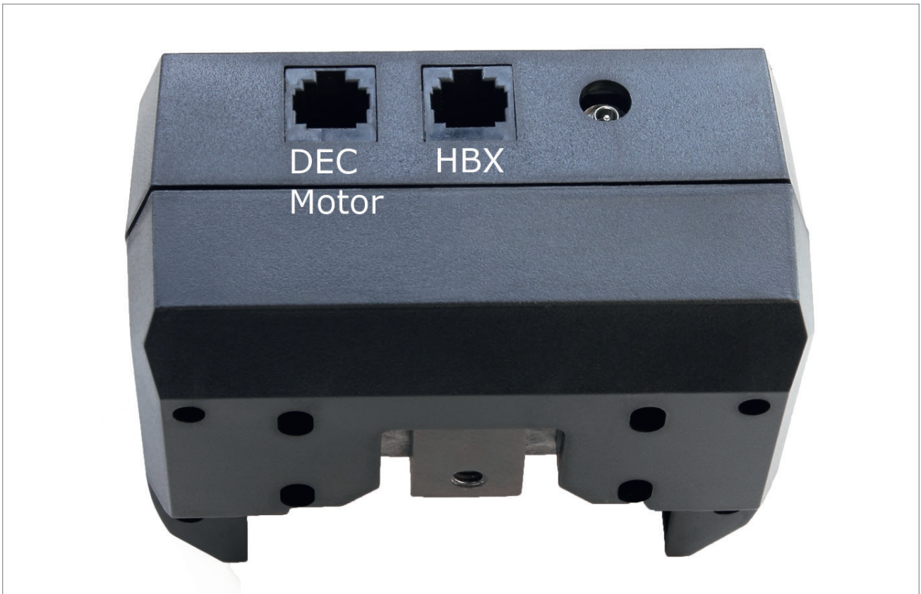
Fig. 1c: Control-Panel of DEC Motor
