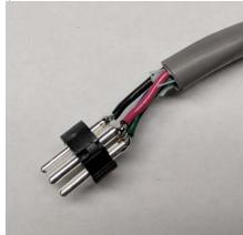
2. Insert the plug to the chasse with two slots aligned to the spring reeds and two pins with wider separation on top of the chasse with alignment notch. Push the plug all the way in.
