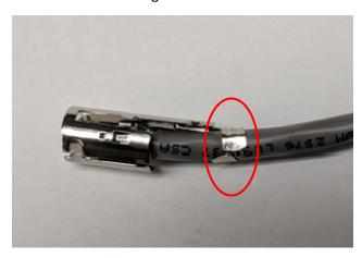
4. Insert the black spring stop ring from the wire end and align two studs along to the spring reeds.
