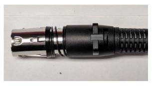
Slide the bottom plastic outer case from the pin end. Align the flat sides too each other and push them together. You should hear the click sound.
