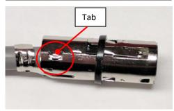
6. Slide the spring on to the chasse from wire end.
