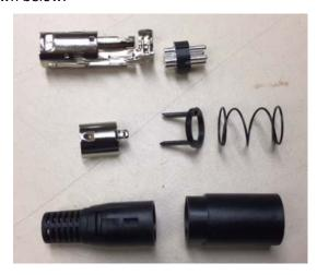
Select a correct wire/wire bundle. Cut to a proper length. Strip the plastic coating outside the wire. Solder them to the short pins on the plug. Please note that 4 pins on the plug are NOT placed uniformly. (see 2)
