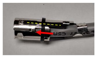
5. Insert the locking piece. Make sure three tabs are locked in position.
