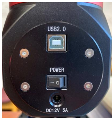
Figure 2. CEM40 Power Panel on Rear of RA axis
