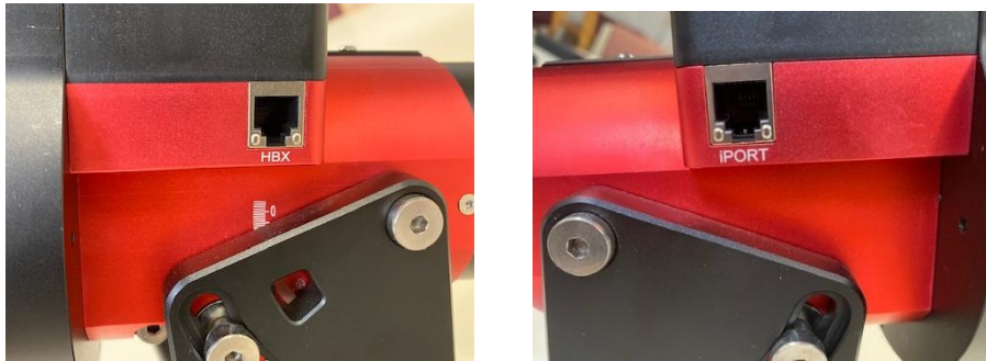
Figure 3. Ports on a CEM40 main board
