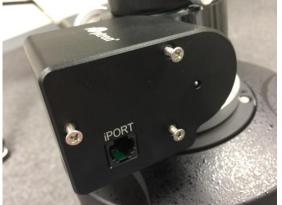
7. Connect the eFocuser to the mount use supplied 6P6C cable (same as the hand controller cable.) One end to the iPORT on the eFocuser. The other end to the PORT (or iPoat) on an iOptron mount.
