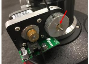
4. Loose four screws that hold the motor in place so you can move the motor shaft close to the eFocuser pulley. Wrap the belt on motor shaft first. Then put the belt onto the eFocuser pulley. You may turn the pulley while install the belt. Tension the belt by push the motor away from the focuser pulley while tightening the motor screws.
