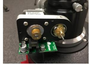
3. Put the eFocuser pulley onto the dual-speed focuser tuning shaft. Tighten the set screw to secure it onto the coarse tuning shaft.
