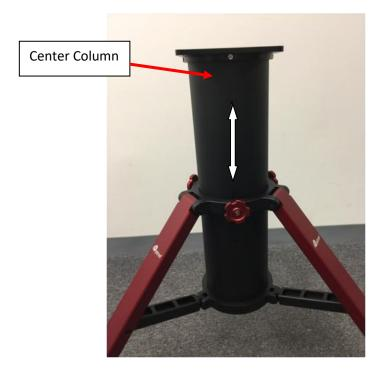
4. Adjust the individual feet to level the pier. Then tighten the feet locker by turn it upward to jam the leg.
