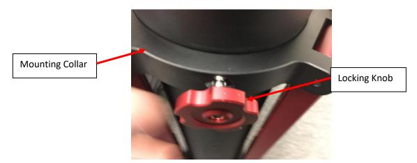
3. Move the Center Column up or down to desired height where there is a hole on the Center Column. Lock the Locking Knob to secure the pier.
