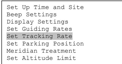
The mount will determine the tracking rate automatically. The tracking rate can be adjusted manually using “**Customer Rate**”. The adjustment range is from 0.9900X to 1.0100X of sidereal.
