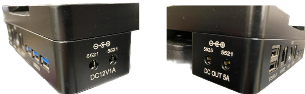
Figure 6. Power output sockets
