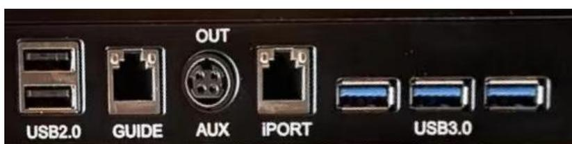
Figure 3. CMS Output ports
