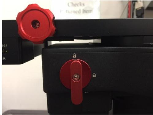
Rotate DEC saddle to exposure two small holes next to DEC **Gear Switch**: one on the top cover (3mm diameter), one on the side (5mm). There is a **set screw** inside the 3mm hole to lock the **gear adjustment screw**, which is inside the 5mm hole.
