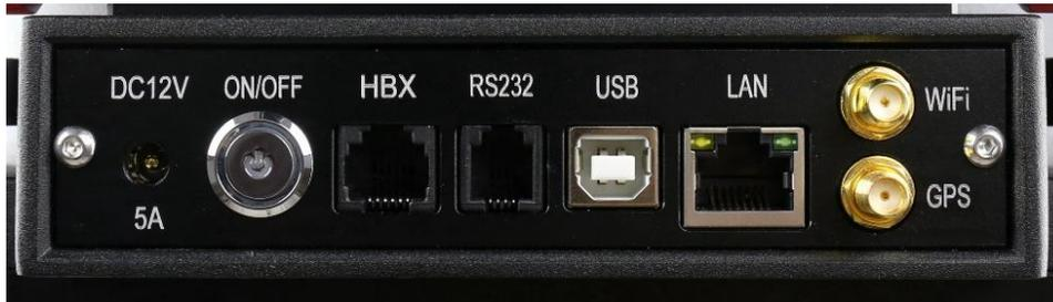
Figure 2. Ports on a CEM120 mount base
