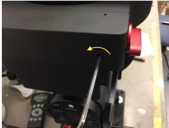
If the motor stalls or the mount does not tracking smoothly, most likely the meshing is too tight. You may loosen it by about 1/8 turn (**or less for tracking**). **Tighten the set screw to LOCK the gear screw (important)**, then test the mount. Adjust again if needed, but no more than 1/2 turn in total.
