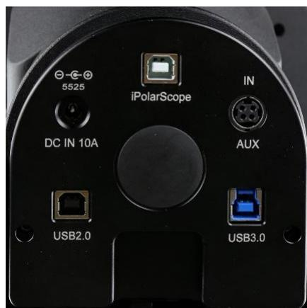
Figure 7. Cable Management System Input Panel
