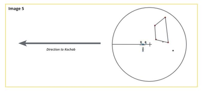
Now clamp the RA-axis again. Then adjust the polar altitude and azimuth settings for the RA axis on the tripod head so that the polar star comes to rest on the Polaris mark when looking through the polar finder. Thus we now have the actual north celestial pole exactly on the centre mark of the pole finder, with which the mount is perfectly aligned.
