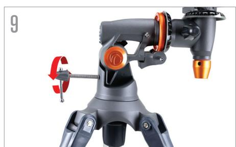
Thread the latitude adjustment screw into the equatorial mount until the screw is touching the inside of the mount.
