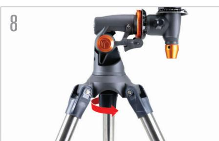
From underneath the tripod mounting platform, thread the mounting nut into the threaded hole on the bottom of the equatorial mount.
