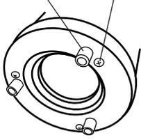
If you see 3 large nuts protruding from the back of your telescope and 3 small Phillip's-head screws besides them, the Phillip's-head screws are the locking screws and the large nuts are the adjusting screws.
