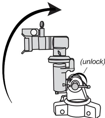
Unlock the altitude lock knob. Set the angle to local altitude.
