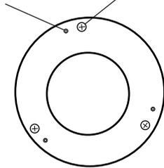
If you see 3 hex bolts and 3 Phillip's head screws, the hex bolts are the locking screws and the Phillip's-head screws are the adjusting screws. You will need an Allen wrench to adjust the locking screws.
