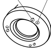
If you see 6 Phillip's-head screws but 3 protruding from the back of your telescope, the 3 protruding screws are locking screws and the ones next to them are adjusting screws.
