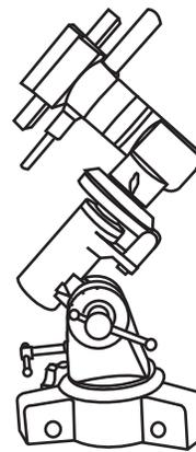
Tighten altitude, DEC and R.A. knobs.
